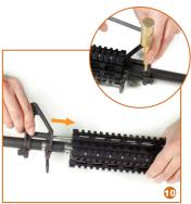
10. Put back the Front Sight with Gas Tube. Replace the two pins to lock the Front Sight to the barrel.
