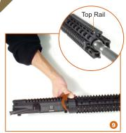
9. Fit the free floating handguard mount onto the barrel nut, and make sure that the top rail of the mount is aligned well with the flat top and that the four alignment pins go into the through holes on the barrel nut. Turn the Locking Cap clockwise until the free floating handguard is locked with enough tension. Use a strap wrench to tighten the Locking Cap and
