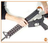
12. Put back the bolt assembly and the lower receiver and stock assembly.
