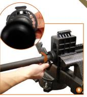
8. Fit the free floating barrel nut on the upper receiver, and tighten it with enough tension. Make sure that one of the through holes on the barrel nut is aligned well with the hole on the upper receiver for the gas tube to pass.
