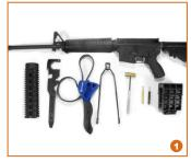
1. Prepare the rifle, the mount and necessary tools (a hummer, a puncher, a strap wrench, a vise, an AR15 upper receiver vise block. an AR15 handguard removal tool, an AR15 barrel nut wrench, etc.). Set up a comfortable working environment.
