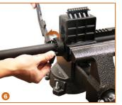
6. Clamp the upper receiver on a vise with an AR15 upper receiver vise block. Loosen the barrel nut by turning it counterclockwise with an AR15 barrel nut wrench. Take out the original barrel nut and the delta ring assembly.
