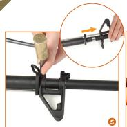
5. Place the barrel on a well padded flat surface securely. Punch the two pins at the bottom of the front sight out with a hammer and a puncher. And, remove the Front Sight with Gas Tube, and take out the Front Cap.
