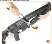
2. Remove the original plastic handguard with a handguard removal tool.
