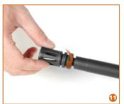
11. Install the Flash Hider on the Barrel.
