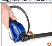
4. Remove the Flash Hider by turning it counterclockwise with a strap wrench.
